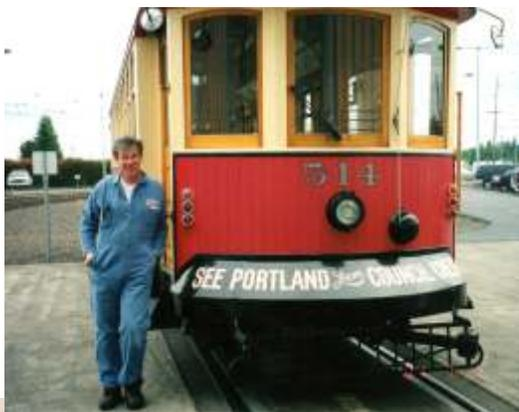
Above: Modified Gomaco Vintage Trolley #514 by adding turn signals, brake lights & mirrors to be used on Portland Streetcar Line. July, 2001.
