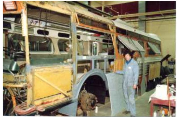
Flexible Bus #435 was involved in a head-on collision with an automobile. The fender well was re-built by Dave in 1981 when no body parts of this kind could be purchased.
