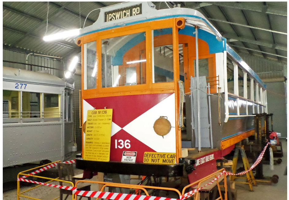
Newly painted Brisbane Tramways No. 136 is seen at the Brisbane Tramway Museum ready to be placed back on its bogeys and rewired (Brisbane Tramway Museum).
