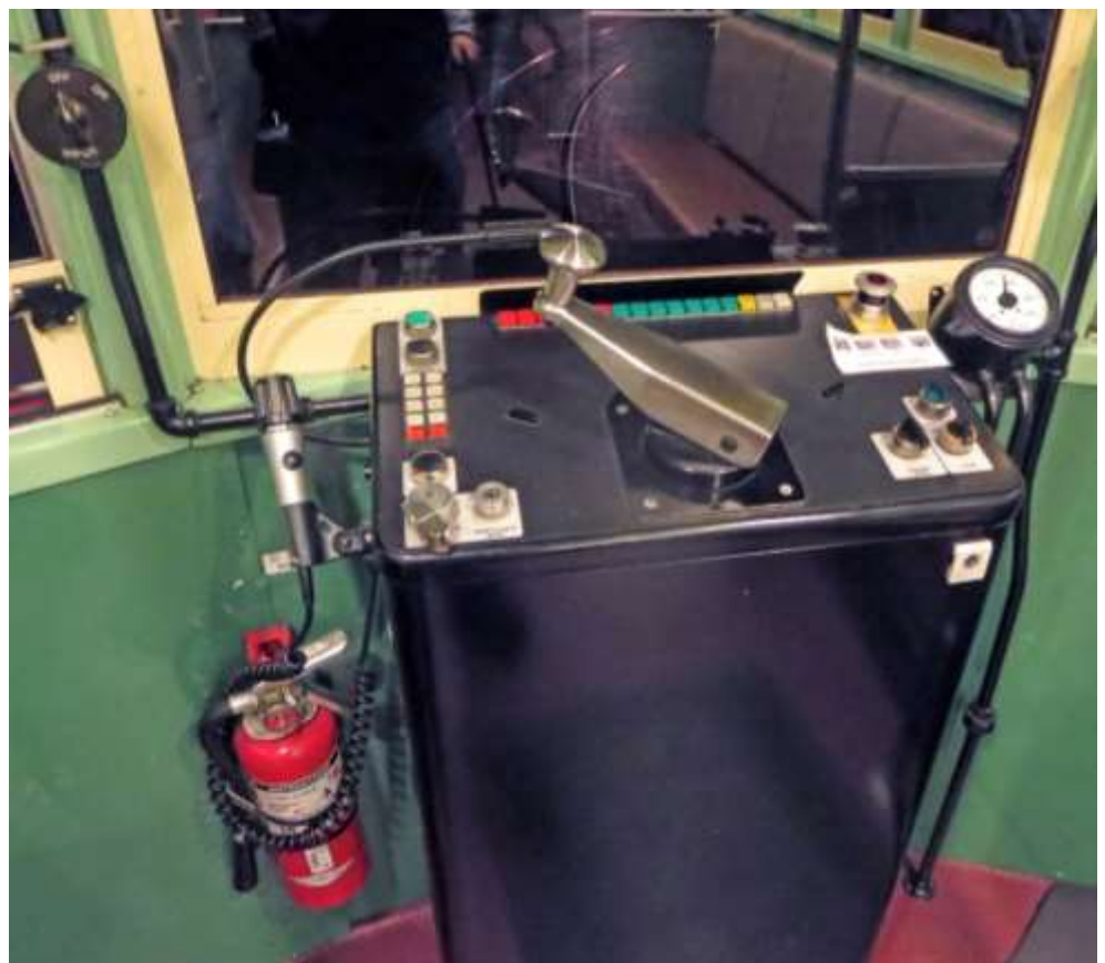
The operating controls in Disney's Red Cars look very similar to authentic controllers, with some changes including a gauge for voltage. (Mark Kavanagh photograph)
