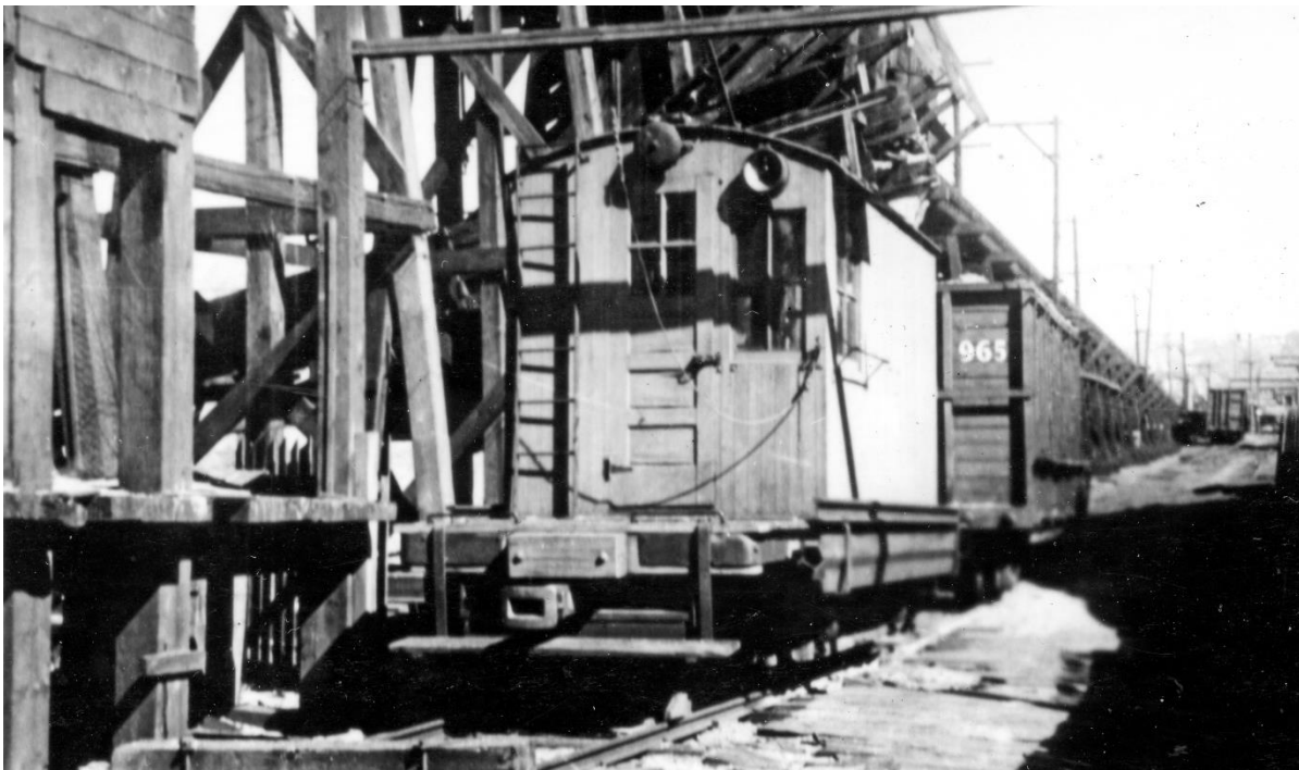
Narrow gauge single cab motor 916 waits while sawdust is loaded into box-sided flat 965 at the Eastern & Western Lumber Co. mill on NW 21 st Ave. This would be hauled to nearby Station E for fuel. Motor 916 is included here because it was similar to No. 914, the sand car described in the article above. No pictures of the sand car have been found.
