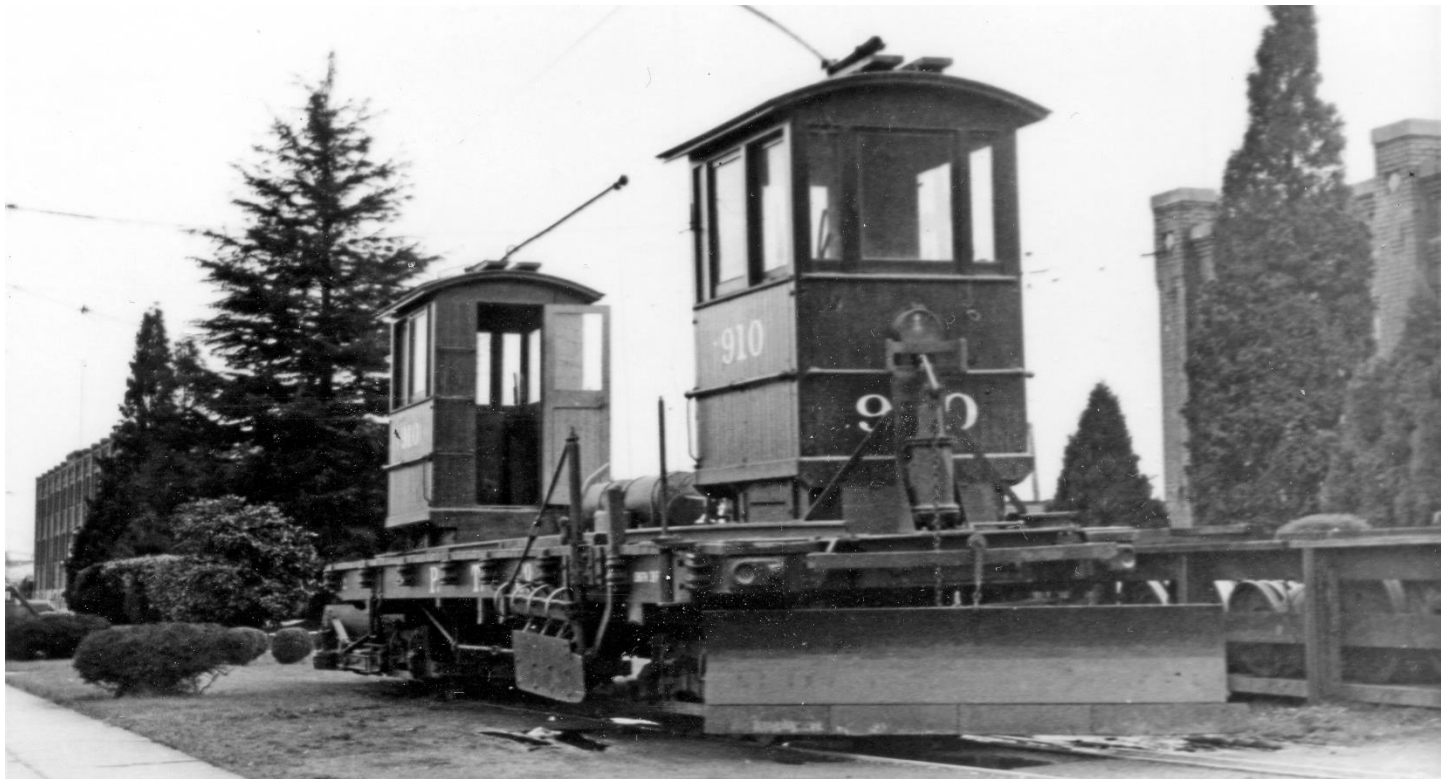
An 8-foot steel shear plow is clearly seen in this photograph of two-cab construction motor No. 910 at the Center Street shops.
