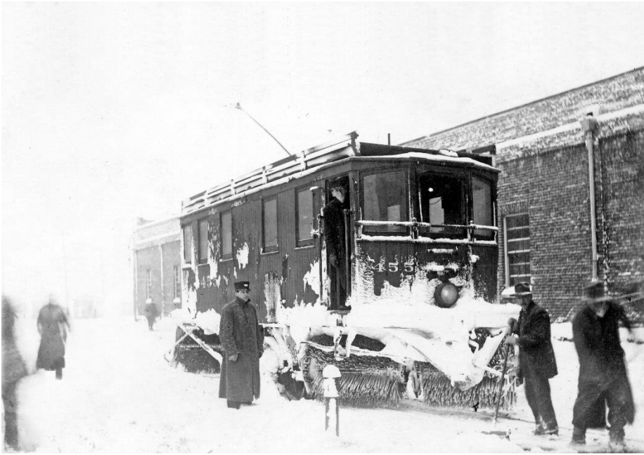
Standard gauge snow sweeper No. 1455 is clearing track adjacent to the Sellwood Car barn in January 1916. Also known as "The Broom," this historic vehicle was built by McGuire in 1899. Portland's oldest surviving trolley is preserved at the Oregon Electric Railway Museum.
