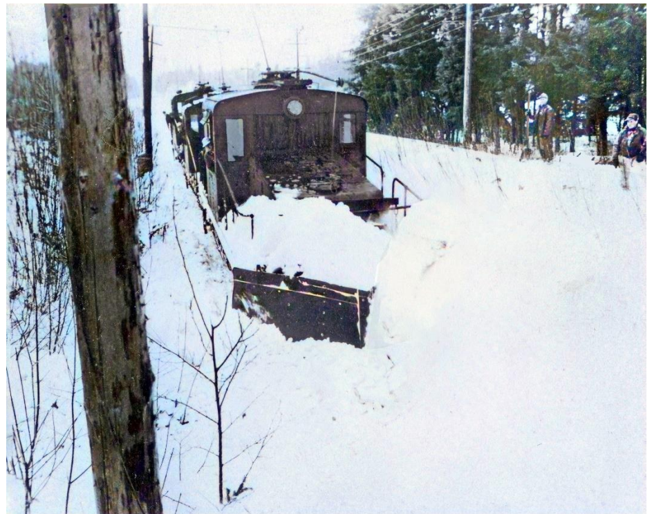
1925 vintage freight motor 1413, seen leading two other electric locomotives on the private right-of-way near the former Sellwood Car barn during a January 1950 snow storm, was the only steeplecab equipped with a pilot plow during the later years. (Colorized by the author)
