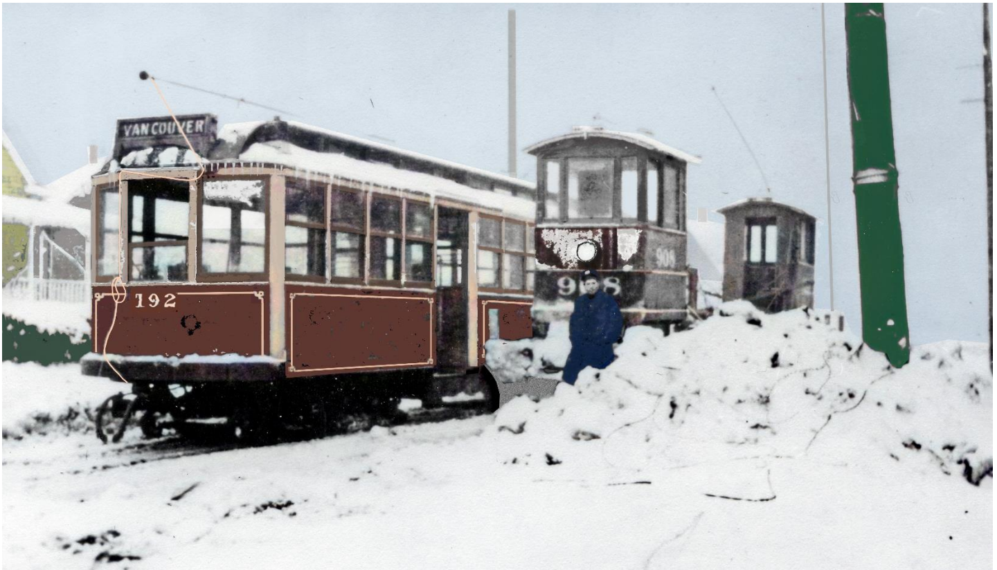
1904 vintage two-cab motorized flatcar No. 908 was equipped with a plow and regularly assigned to winter snow removal. It is seen here on N.E. Union Ave. (now MLK Blvd.) next to "Vancouver" class combine 192, which could also assist since it was equipped with Root snow scrapers. Car 192 was built in 1907 and retired in 1939. Construction motor 908 was retired in 1943.
