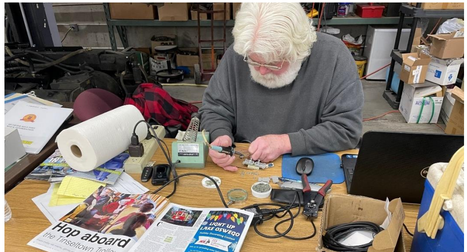
Kevin Reilly building a wire harness to connect a laptop computer to the Vehicle Control Unit in Vintage Trolley No. 514. Note The Lake Oswego Monthly Magazine for December with an article on the "Tinseltown Trolley." (Dave Rowe photograph)
