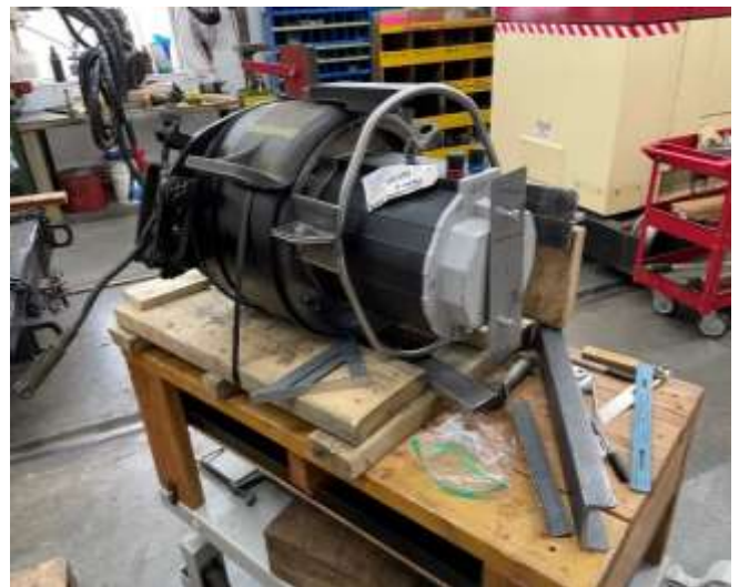
Dave Rowe is designing a motor retention cage so that if a motor mount broke it would be held in place and not cause a possible derailment. (Dave Rowe photograph)
