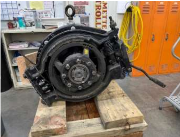
One of the old shaft brakes has been mounted on a new AC motor. The shaft brake will serve as a parking brake for the battery-powered Vintage Trolley. (Dave Rowe photograph)
