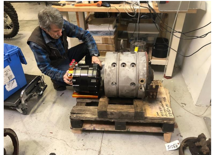
Bob Simpson is aligning the new AM Racing ac electric motor to the original DC motor housing. The shell of the old motor will be adapted to mount the new AC motor. The old DC motor weighed over 700 pounds while the new AC motor will weigh less than 100 pounds and puts out about the same house power.
