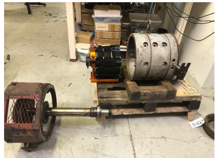
The old motor and internal shaft will be cut shorter and connected to the new AC motor. The trolley shaft brake assembly will remain the same.
