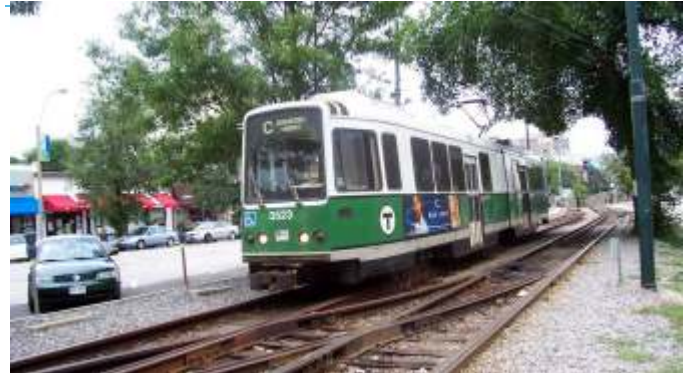
Boeing Vertol LRV car, one of an original 50 cars (later expanded to 175) built for Massachusetts Bay Transportation Authority (MBTA) in Boston. The articulated light rail vehicles entered revenue service on Dec. 30, 1976, on Boston's MBTA Green Line "D" Branch. By March 1, 1982, 114 LRVs were in Boston's MBTA active service fleet and Boeing Vertol delivered the last LRV in 1983. The MBTA's last revenue run of a Boeing LRV was March 16, 2007. However, the MBTA continued to operate three LRV work cars. Shown here is Boeing Vertol USSLRV #3523 in service for the MBTA on the Green Line "C" Branch, bound for Cleveland Circle, in 2005. This view shows the roof-mounted air-conditioning units and bi-fold doors added by MBTA in place of the original equipment.
