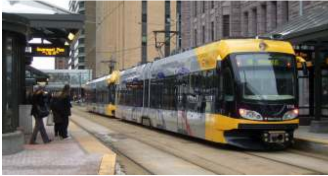
A two-car train of 100-series Bombardier FLEXTY Swift vehicles in downtown Minneapolis on the METRO Blue Line Hiawatha Line at Government Plaza - Metro Transit station, part of a fleet of 27 cars that began operation in June of 2004. In 2010, the Metropolitan Council contracted with Siemens Industry Incorporated to build up to 109 S70/Avanto light rail vehicles, with the first vehicle arriving in September 2012. Most are intended for the Green Line which opened in 2014, and is to be expanded from Minneapolis to Eden Prairie along the Southwest Corridor in 2018, though the initial vehicles were used on the Blue Line as part of that route's three-car expansion project.
