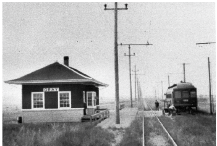
Looking south with the OE Gray station on east side of tracks. The Jewett combines #52, 53 & 56 had been converted to double end operation on the Corvallis and Woodburn branches to eliminate turnaround trackage. The Corvallis train will turn right onto the branch line.
