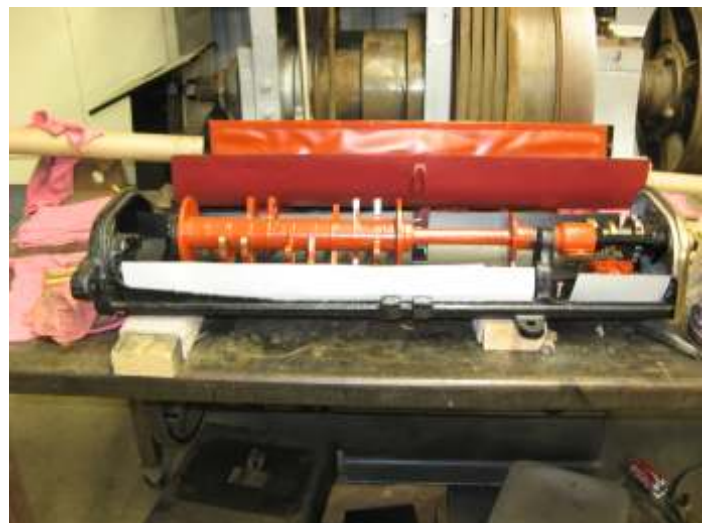
Restoration work on the controller for electric locomotive 254 by John Halls.
