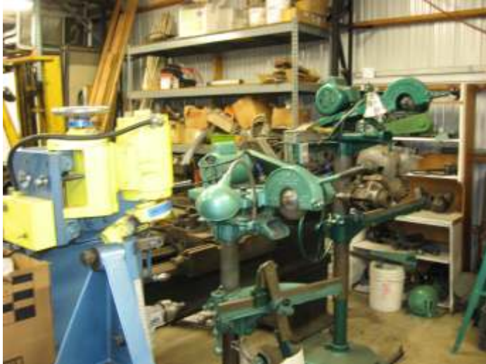
Overall view of new shop. Donated saw filing equipment ready for use in the machine shop.
