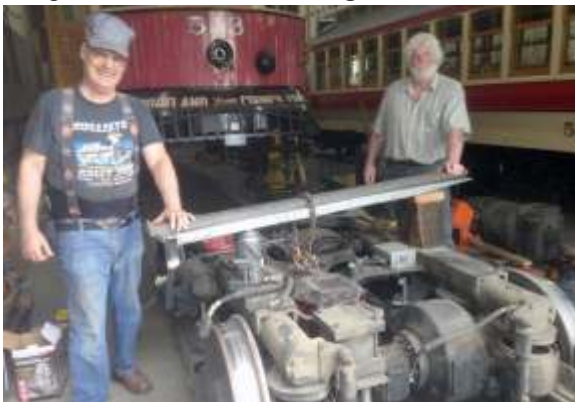
Kevin Reilly working on a modification on VT 513. This modification will allow the trolley to still operate if any of the four traction motors fail.
