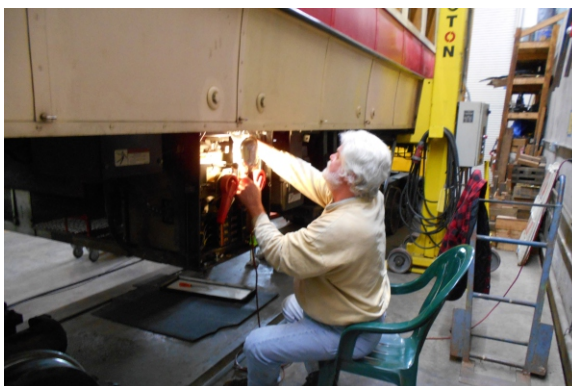
Kevin Reilly working on a modification on VT 513. This modification will allow the trolley to still operate if any of the four traction motors fail.
