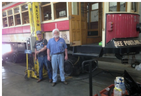
Removing bad motors from VT 513 Steve Mills and Kevin Reilly assisted Trolley Dave in removing two defective motors from VT 513 inside the WST Trolley Barn. The four Macton jacks.
