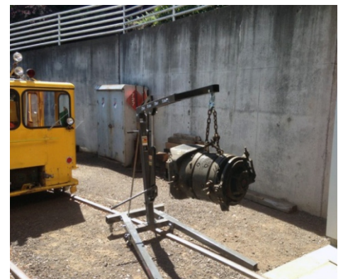
Removing bad motors from VT 513 Steve Mills and Kevin Reilly assisted Trolley Dave in removing two defective motors from VT 513 inside the WST Trolley Barn. The four Macton jacks.
