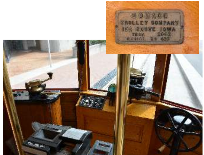
Motorman's position with vintage controller and modern fare collection box. Waiting on Franklin Ave. at Whiting St. station. Also shown is the builder's plaque that is located inside the car.
