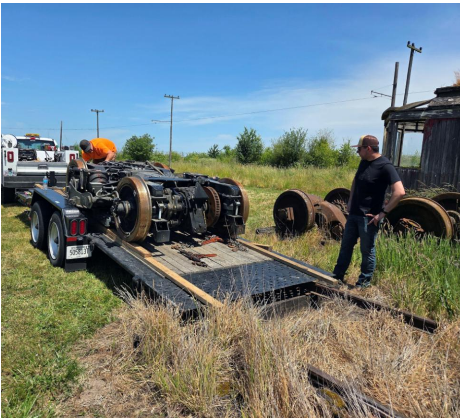
This Type 1 power truck being rolled off a trailer onto tracks behind the Oregon Electric Railway Museum car barn, is one of the larger “parts” we have acquired. (Mark Kavanagh photograph)
