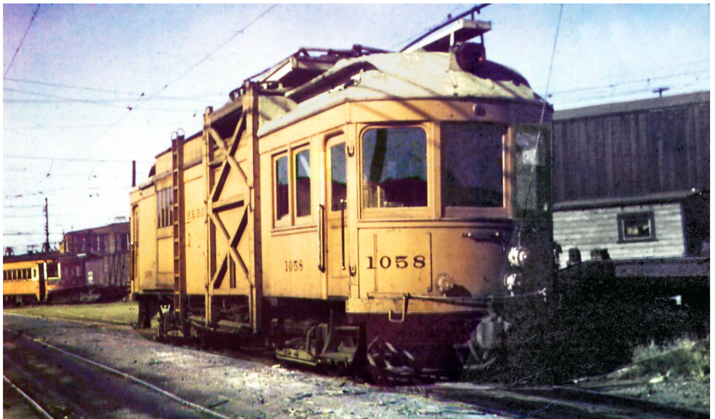
Once beautiful Niles Interurban 1058 survived until the end of service because it had been converted into a line repair car in 1930. It is seen next to a loading dock in East Portland. In the background is one of the two former Fonda, Johnstown and Gloversville cars, 4006 or 4007. In 2019 a much-deteriorated No. 1058 was scrapped in Snoqualmie by the OERHS and its engines, controls, and running gear salvaged for use on No. 1067.
