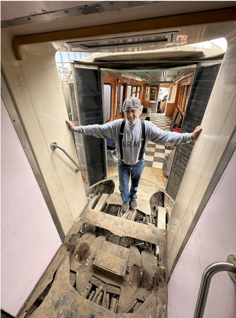
Separation completed at last! All four pins have been removed and Greg stands between the slightly separated A and B sections of MUNI car 1271.
