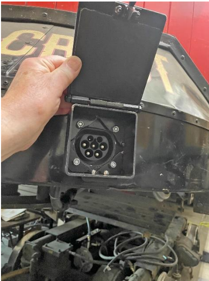
As the battery charging receptacle is installed VT 514 begins to act like a Tesla!
