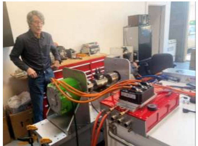
Bob Simpson with the EV Drive dynamometer, the only one in the Pacific Northwest at this time. This unit can handle from 100 to 800 volts as it synchronizes the four inverters to the new AC motors.
