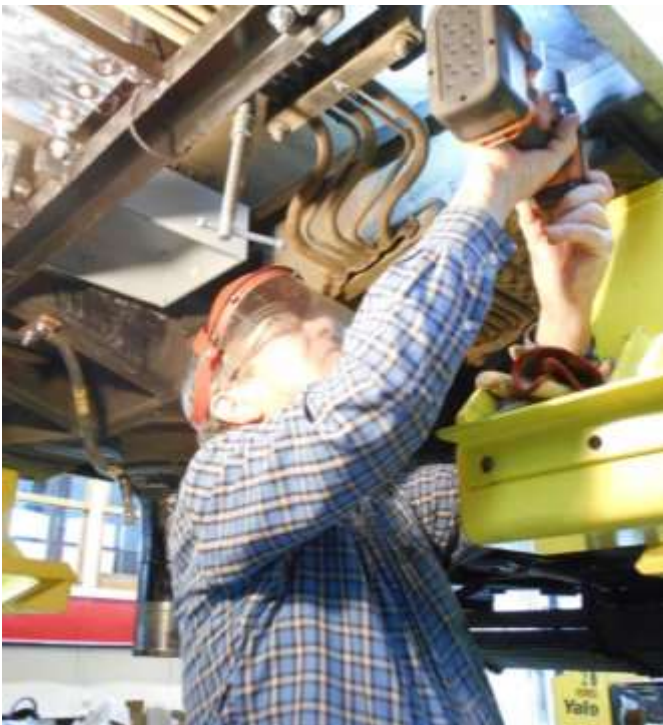
Dave Rowe mounting a support for the four inverter motor disconnect boxes on VT 514.
