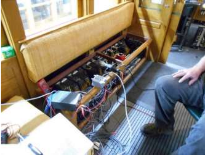
Kevin Reilly made test boxes to check system circuitry for the battery project. He is testing circuits beneath a longitudinal seat.
