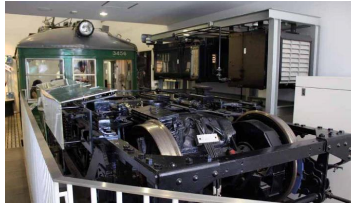
Tokyu Museum: Guest can operate the train from the cab seen in the photo. The control group seen above the trucks would function, and the wheels on the truck would rotate based on operator input.
