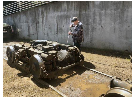
Dave Rowe is pressure washing one of the PCC trucks removed from Trolley 514.
