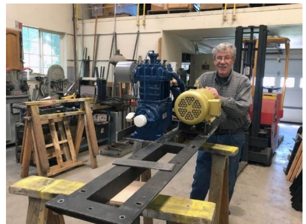
The Quincy air compressor was lowered 3" and mounted on a removable tray to allow for easier maintenance from the original Gomaco M/G designed frame.
