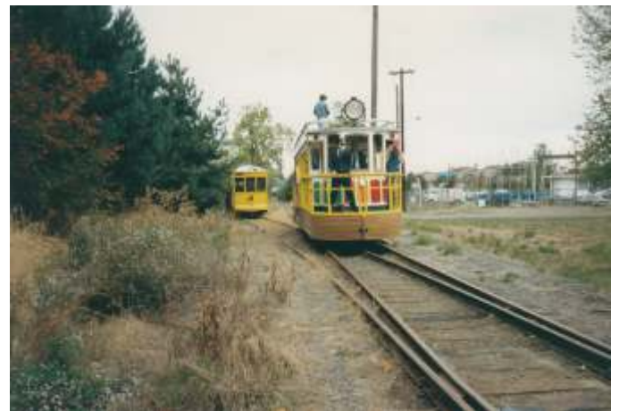
This is a "rare photo" of two streetcars in revenue service at the same time. The location is the WST siding just north of Nebraska St. The date: Sept. 18, 1992. Southbound on the main is car #731, the Blackpool Belle. "In the hole" is San Antonio Car #300. We used the staff-exchange system to avoid mishaps between the two. After the pass, and with staff in hand, I took car #300 out to the main, and proceeded to our northern terminus at Sheridan St. This was the Belle's maiden run, and thankfully, everything mechanical and electrical on both cars performed without attendant problems. Noteworthy is the spotlight atop #731
