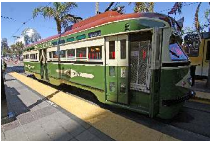
PCC #528 at 12th/Imperial. Note the ADA lift clearly blocking the original front entrance to the car
