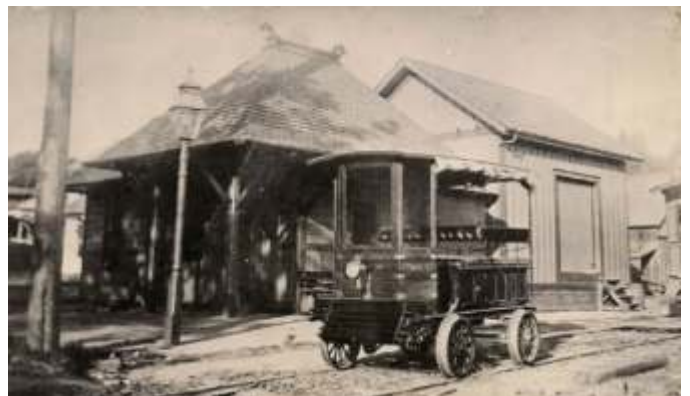
Small town railways sometimes augmented steam or electric trains with gasoline-powered "doodle bugs." The Rogue River Valley Railway pioneered modern passenger service by introducing this eight passenger Fairbanks Auto Car in 1905. It is seen at the station in Jacksonville. The Southern Oregon Traction Company merged the Medford streetcar system and Jacksonville railway in 1916, after which the Jacksonville was electrified joining the already electrified Medford system.
