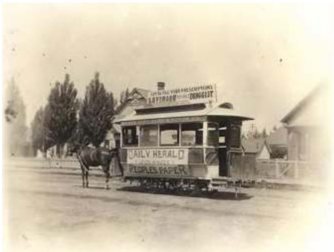
Baker City Street Railway & Motor Company horsecar No. 2 in a residential neighborhood, likely the southern terminus of the line, at Front Street and Auburn Avenue. In spite of the ambitious name, the Baker City operation never converted to electric power. By 1902 citizens were petitioning to have its abandoned rails removed.
