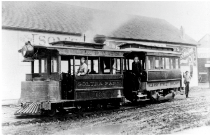
The Albany Street Railway could boast of the first mechanized streetcars in the Willamette Valley outside of Portland. Steam dummy engine No.3, with former horsecar No. 1, pauses on Lyon Street on the new line to Goltra Park in the 1890's.
