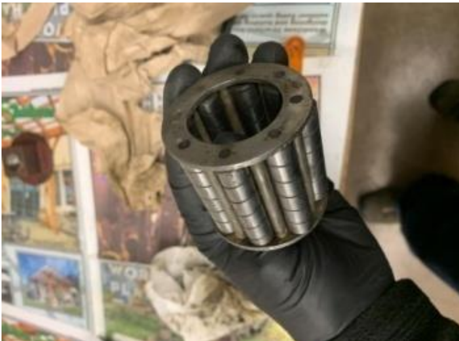
Large wheel bearing removed from baggage cart for cleaning (Rick Lucia photograph)
