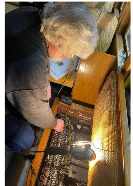
While Dave Rowe was under the car checking wiring Kevin Reilly was at the other end of the wires to verify that they were connected correctly (Dave Rowe)
