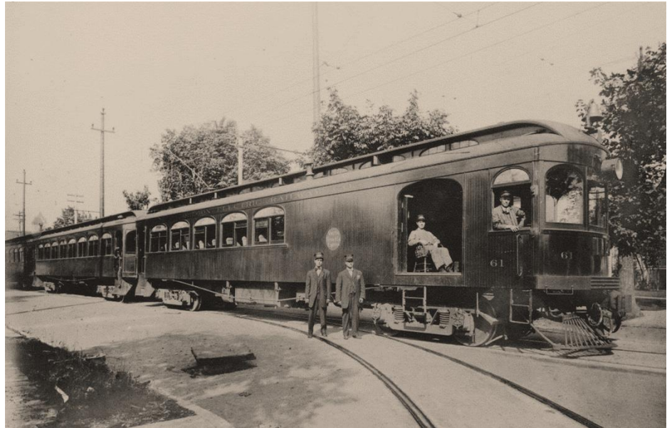
This photograph of Oregon Electric combine No.61 shows it in original Pullman green livery. Car 61 featured a larger express section and smaller passenger accommodation than sister No. 65. Both were built by the American Car Company. (Richard Thompson Collection)
