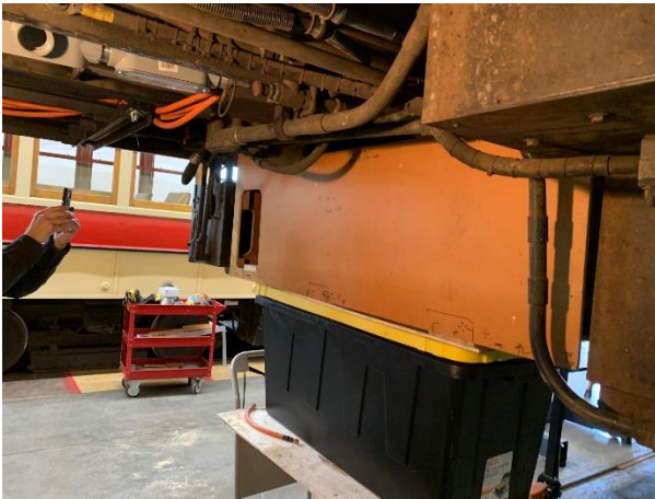
The mock-up battery was raised in place by a lift table.
