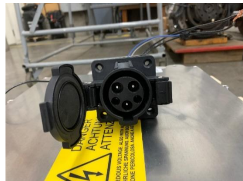
This is the receptacle for charging power into the trolley that will be mounted on the trolley anti-climb bumper. It is an industry-standard SAE J1772 connector, the same type used on domestic Electric Vehicles for a Level 2 charge. It accepts 120 to 240VAC single-phase at up to 75A although is more typically 30A to 50A (7.5kW to 10kW).
