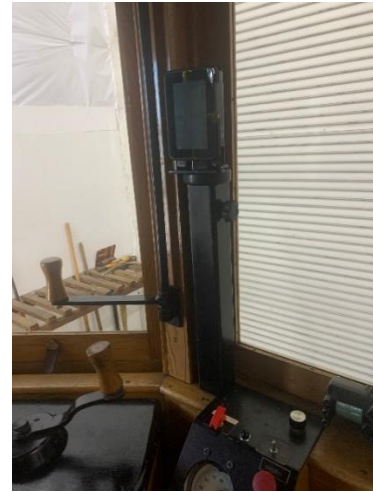
The motorman's display. It is mounted at eye level and is a touch screen similar to a cell phone screen. It will display speed, controller notch, battery health and other information.
