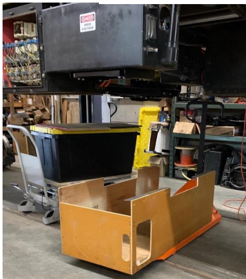
This is a wood mock-up of the battery case that will be installed where the old DC resistor rack used to be.
