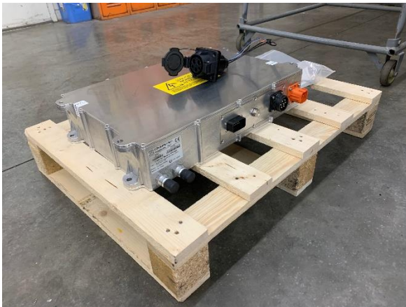
The 11kW battery charger that will be installed on the trolley. The trolley will be charged overnight from a 40 amp 208 three phase wall plug.
