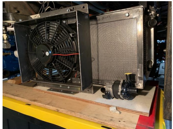
View from the intake side of the radiator shroud. The left side has the screen removed to show the fan. The right side has the screen installed. This screen mesh has proven best to keep cottonwood seeds from the radiator. In the right corner is a coolant pump is one of three.
