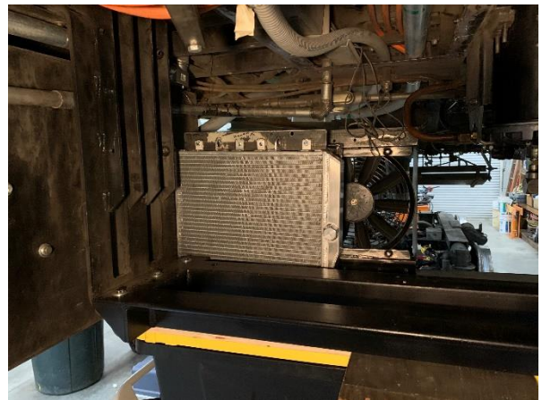
The two radiator mounts front and back still under design. When finished they will be painted with a powder coat. The two radiators will cool four AC motors, five inverters and the battery charger. View of the exhaust side of one installed radiator and the fan without the second radiator.
