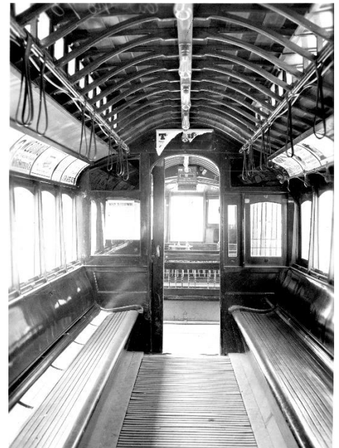
Classic streetcar details in this interior view of No. 78, include clerestory windows, a large metal fare register, advertising cards and standee straps. The "all weather" trolley featured longitudinal bench seating in the enclosed end, and spindle-backed cross bench seating on the open end. The floor was designed for easier cleaning, since dirt fell between the slats.
