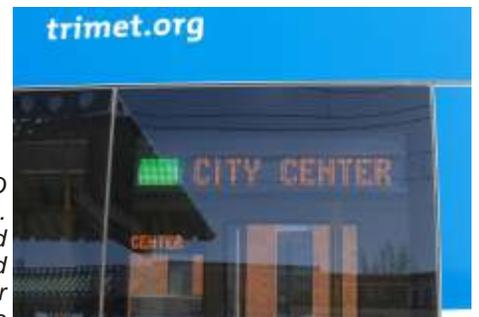
New Type-4 LED destination signs. These are used both on the side and front-rear destination signs as shown. The LEDs can be set to any color. A color square identifies the line.
