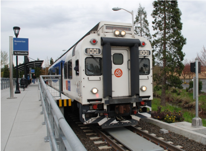
A single car train waiting at the Beaverton Transit Center to return to Wilsonville. When traffic is low, a "train" is a single car, more typically with heavier traffic, trains are a two-car unit back to back. A smaller driver's cab is provided on the B end as shown.
