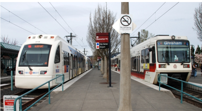
New Type-4 car on the left contrasted with older Type-2 car on the right at the Beaverton Transit Center station
