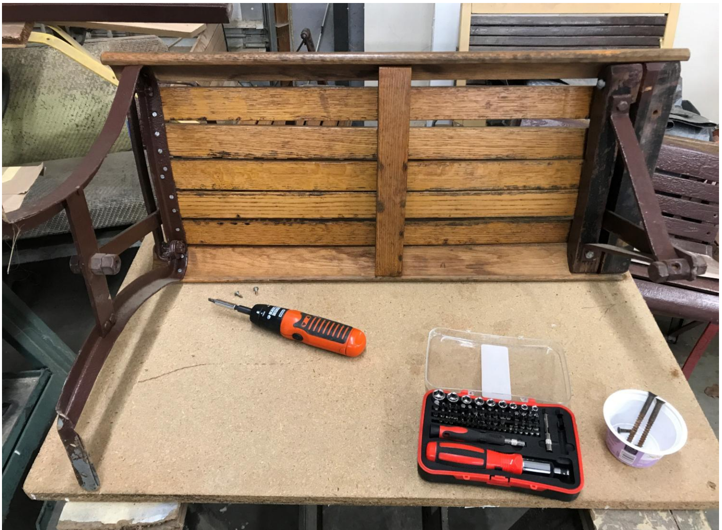
A bench from the upper deck of tram 48 being disassembled for cleaning and refinishing. (Pete Manuele photograph)
