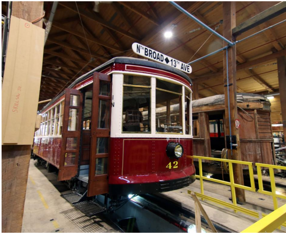
Seen in the ERRS shops, the restoration of Regina Municipal Railway 42 is nearing completion. No. 42 is an all steel car built by Canadian Car & Foundry in 1928. (Mark Kavanagh photograph)
