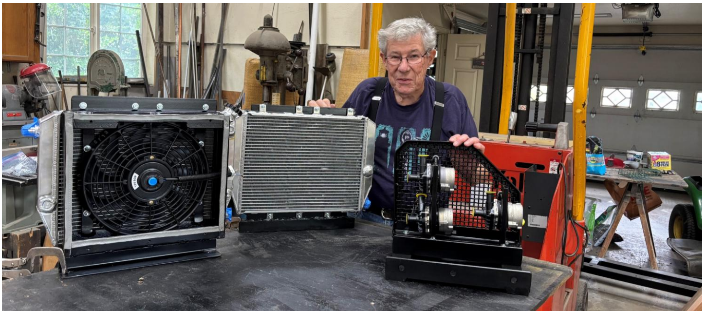
Dave Rowe is displaying several components made in his shop for the Trolley 513 Battery Project. On the left is a 12-volt fan mounted on a radiator. At center is the second radiator from the back side, and on the right are three coolant pumps. Two pumps are for both truck traction motors and inverters. The third pump sends coolant to the battery charger and auxiliary inverter. The challenge is to mount these in a limited area.
