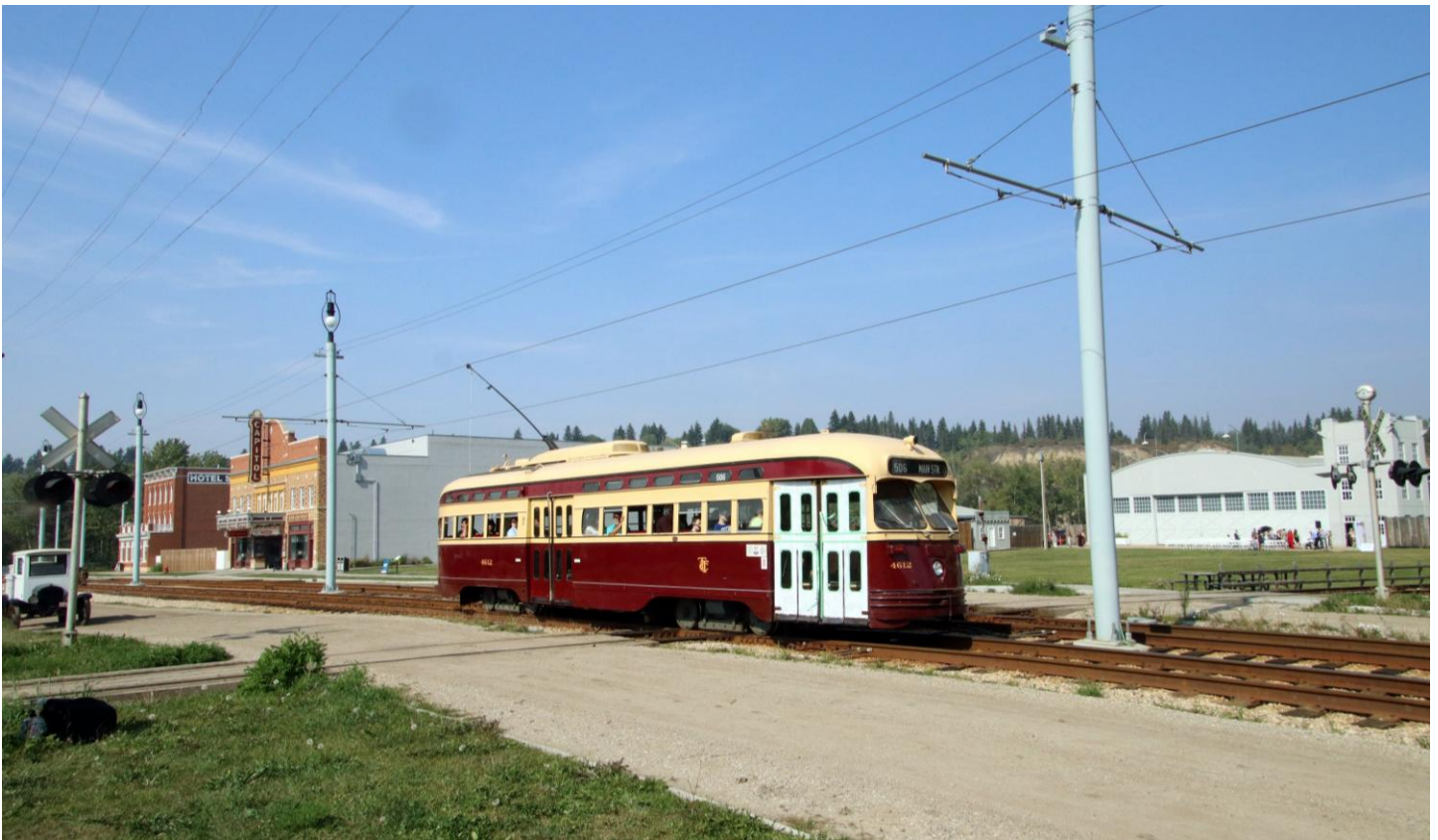
Toronto PCC No. 4612 is a 1951 product of the Canadian Car and Foundry. The Toronto Transit Commission donated it to Fort Edmonton Park in 1995, and it was returned to service two years later after regauging with Melbourne trucks. (Mark Kavanagh photograph)
