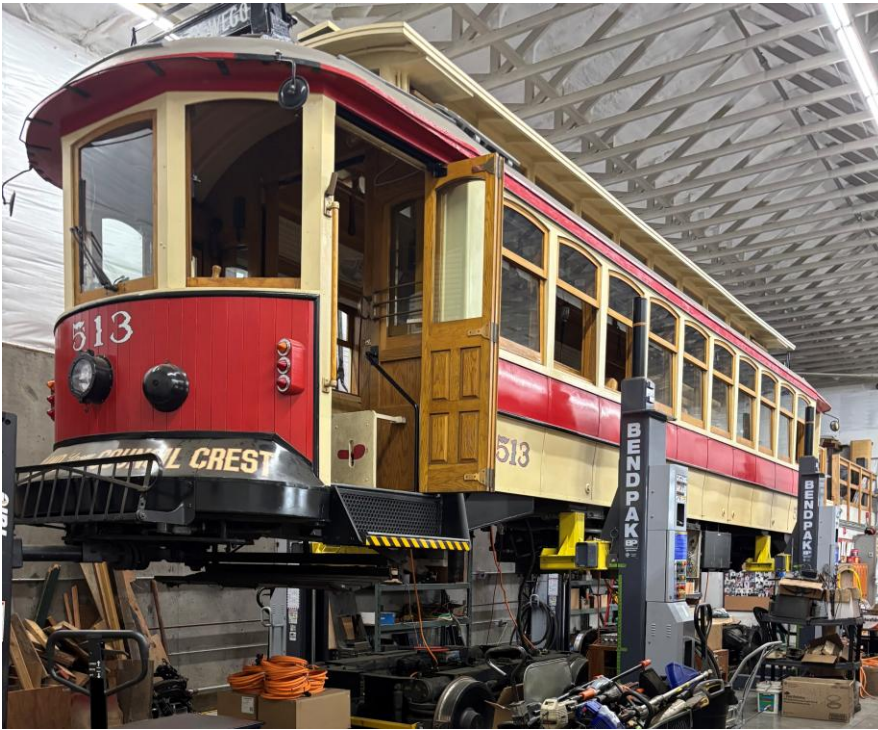
Trolley 513 has been lifted with heavy duty jacks for installation of new electrical equipment necessary for conversion to battery operation. This includes many feet of conduit with thousands of feet of wire inside. The picture at right shows the 80 KWh battery. (Dave Rowe photograph)
