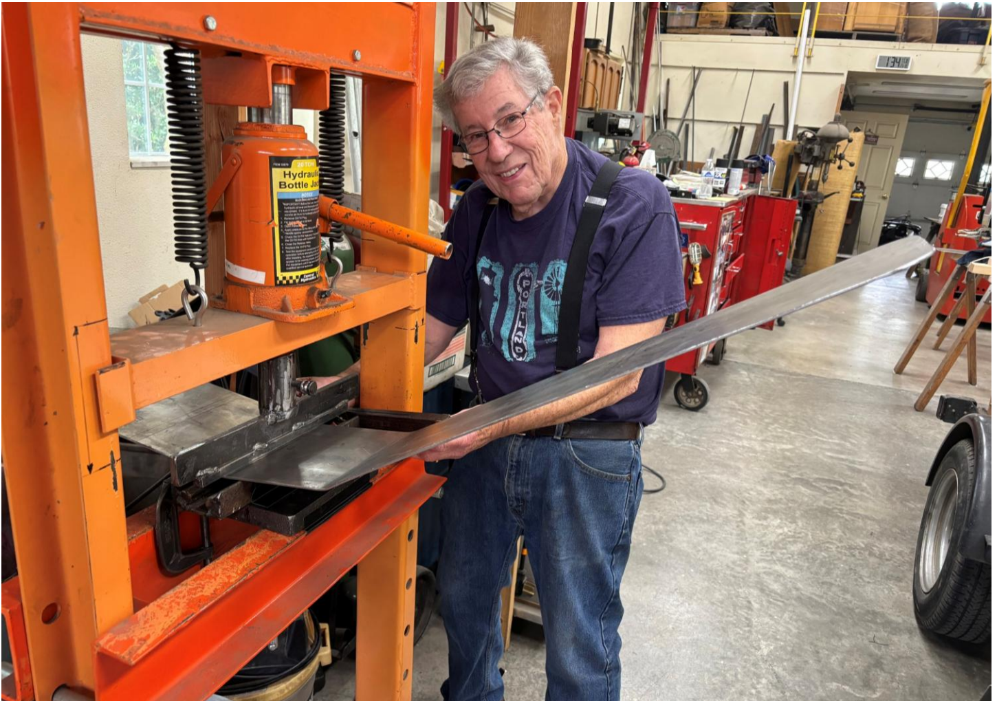
Dave Rowe is using a metal brake made in his shop to make the first bend in a fender/splash shield for car 513.
