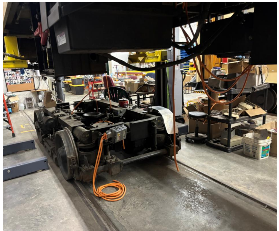
The silver component with the orange wire seen in this photograph is a newer model PM-250 inverter. It will be used instead of the older style PM-150, which experienced problems on sister car 514. The invertors are made at Cascadia Motion in Tualatin. (Dave Rowe photograph)
