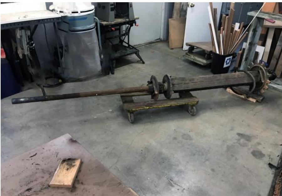
One of the two brush assemblies from snow sweeper No. 1455, "The Broom," is being disassembled in the shop. (Pete Manuele photograph)
