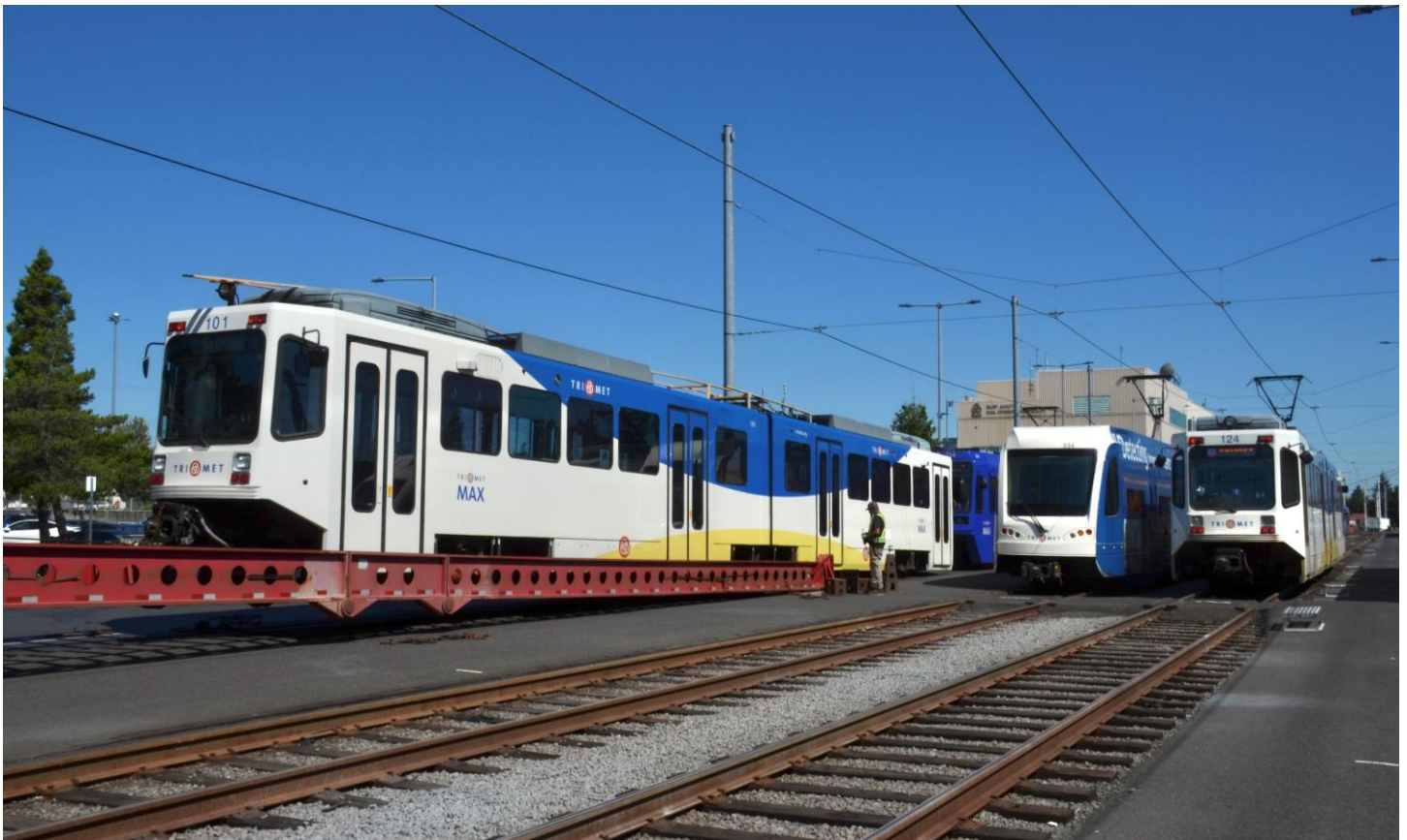
Car 101 being loaded onto the trailer in the main yard at TriMet's Ruby Junction maintenance and operations facility, in Gresham, on July 16. It is being pulled by a cable attached to a winch at the other end of the trailer. Car 214 had moved No. 101 into position just short of the trailer. Cars 534 and 124 are parked at right. No. 101 was moved to the museum the next day (Steve Morgan photograph).
