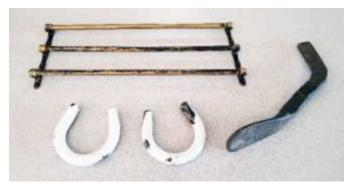
Clockwise from top: Brass rod bulkhead window guard, sander pedal, and enameled standee strap handles. (Mark Kavanagh)
