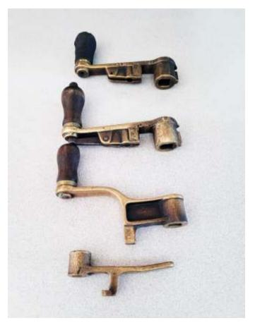
Top to bottom: Removable brass handles for electric brake controller, controller, and reverser. (Mark Kavanagh)
