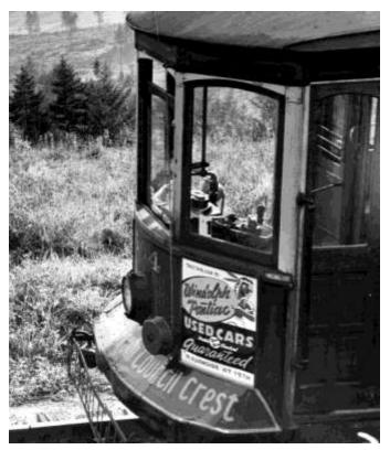
The dual controllers and window guards on Council Crest cars can be seen through the window of No. 504 in this view on the upper loop taken on August 9, 1949.
