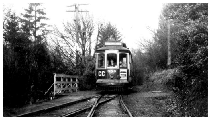
Council Crest Line train one, car 506, is seen outbound, entering the upper loop on Council Crest. Note the United States Electric Company block signal mounted on the pole to the left. Portland was the only city in the West to use this type of signal. (Bill Hayes Collection)
