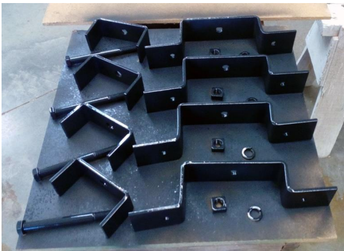
Roof support brackets
