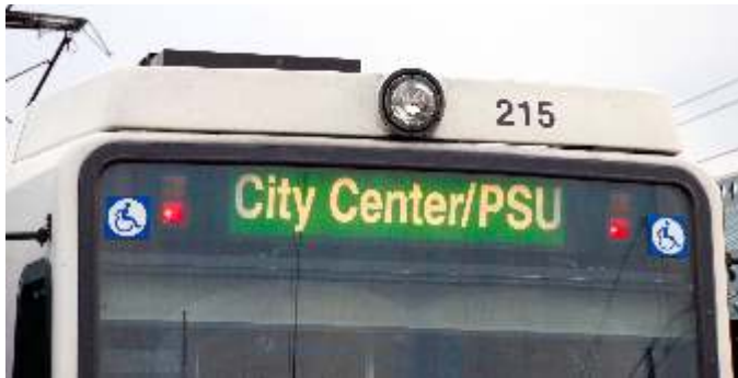
Close-up of MAX Type 2 rollsign on a Green Line run. Steve Morgan
