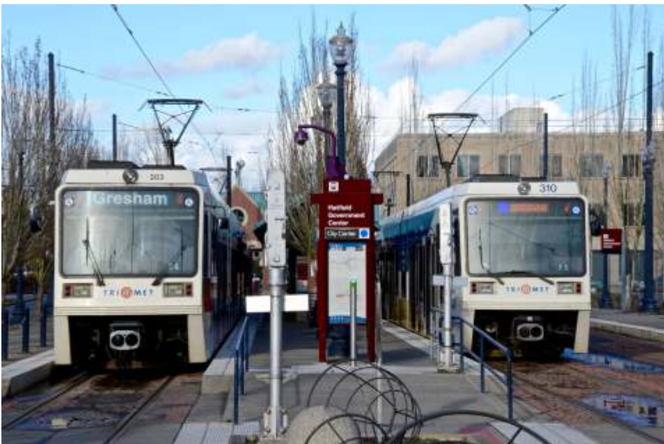
In September 2016, TriMet completed a two-year program to replace the rollsigns in its 105 older LRVs with LED signs. This photo shows two Siemens SD660 cars at the MAX Blue Line's Hillsboro terminal in January 2016. Car 203 (left) still had rollsigns at that time, while No. 310 had been retrofitted with LED signs.
