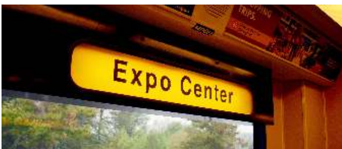
The destination sign display for "Expo Center", on the side rollsign in a Siemens SD660 LRV northbound on MAX Yellow Line. This is the interior side of a two-sided signbox, which displays the identical reading on the exterior and interior of the light rail car. Steve Morgan
