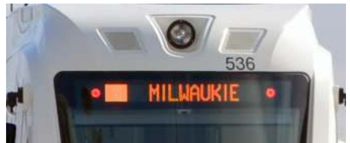
A different type of LED sign on a Type 5 Siemens LRV on the Orange Line. Wayne Jones
