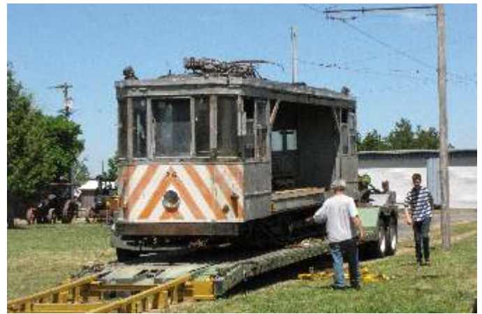
Car 26 is a single-ended "works" tram. It was built in 1934 as car #1085. It was converted to work service around 1975.
