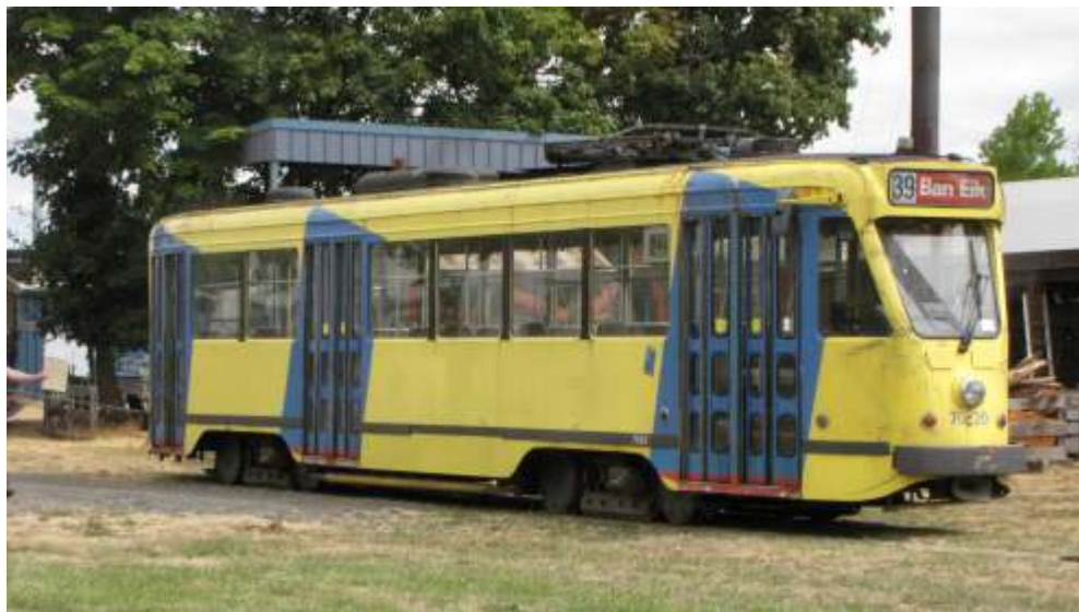
Car # 7020 is a Brussels PCC built in 1952. It is very similar to a US PCC with the exception of its narrower body (although standard track gauge).
