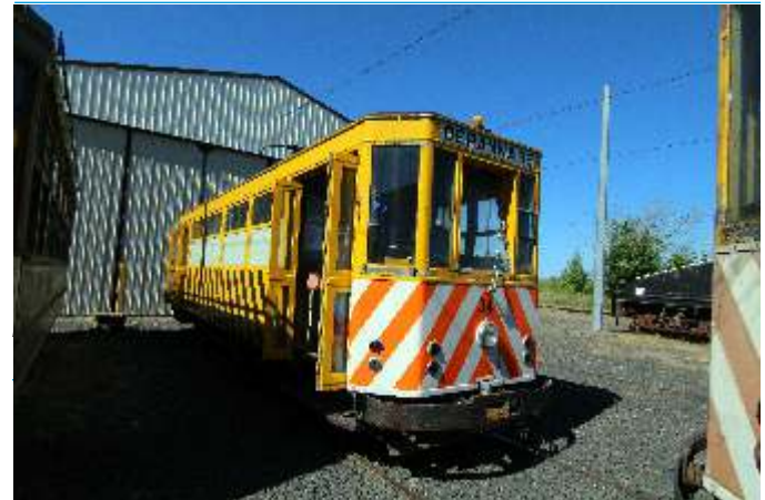
Car # 34 is a double-ended "works" tram. It was built in 1934 as car # 1290 and converted to work service in 1971.
