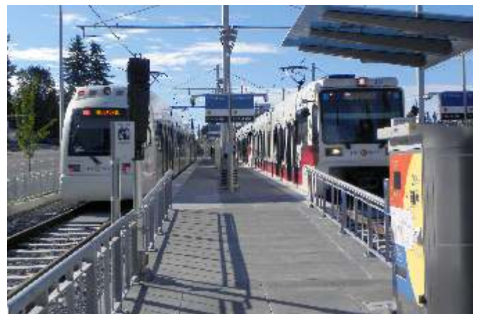
SE Park Ave station with Siemens LRVs type 4 on the left and type 2 on the right.
