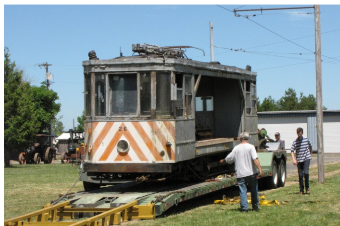
Car 26 is a single-ended "works" tram. It was built in 1934 as car #1085. It was converted to work service around 1975.
