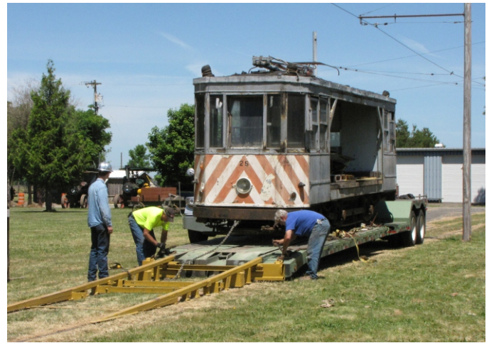
Unloading each car was a multi-step painstaking operation. Here attaching the roll down ramp.
