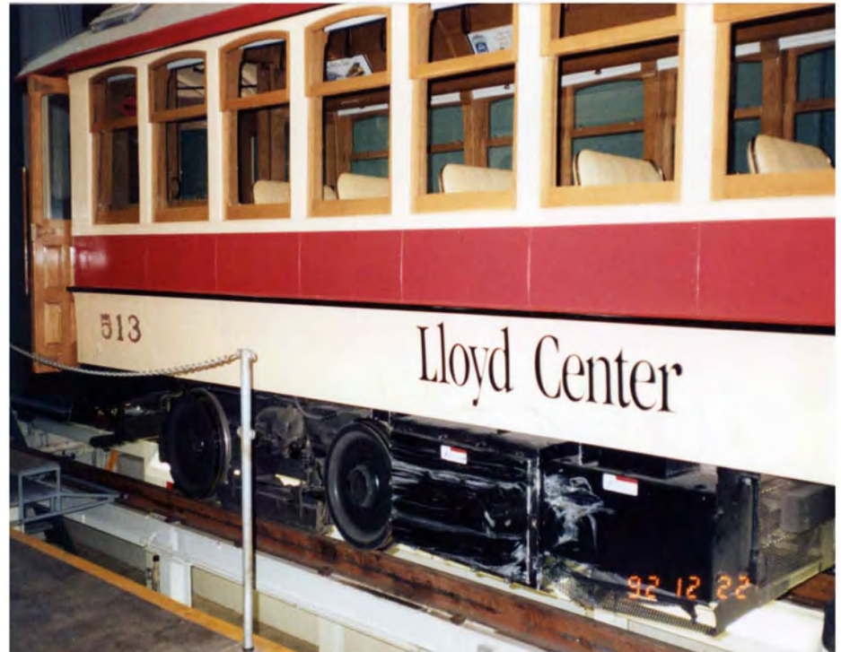
Light hit and run damage is evident on the motor contactor and inverter panels and resistor grid screen beneath car 513 in this view taken after the trolley was moved to Ruby Jct. under its own power. The car was returned to service after approximately 60 hours of repair (Jack Goetz photo).
