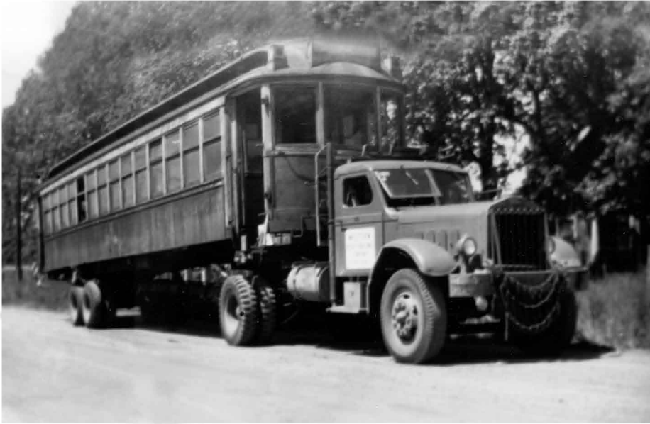
A chain drive Sterling log truck makes easy work of hauling recently retired interurban 1094 to an unknown new home in this 1946 snapshot taken by member Jack MacDougal near Estacada (Jack MacDougal photo).
