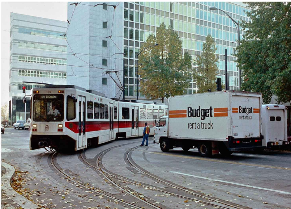
The Vintage Trolley spur on N.E. 11th is also usable by light rail cars, although such use will be rare. On Nov. 15, 1991, during clearance testing, car 107 became the first LRV to enter the spur (Steve Morgan photo).
