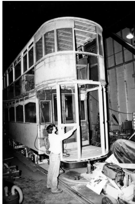
Museum Director Greg Bonn is seen installing support posts on No. 48 during the Fall of 1984. Metal pieces have been bored and counter sunk for placement on the car side and interior and exterior priming begun on this double-deck tram from Blackpool, England. (Bud Statton photo)
