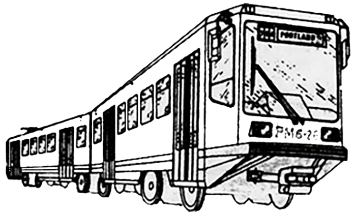
Six-axle, articulated car to be built by the Bombardier Corporation of Quebec, Canada for Portland (Tri-Met sketch).
