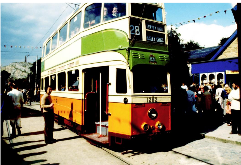
Glasgow No. 1282 was part of a group considered to be among the most luxurious of tramcars ever to have entered public service. It was built by Glasgow Corporation in 1940 and features tapered ends that enabled it to negotiate the city's sharp curves. (Richard Thompson photo)
