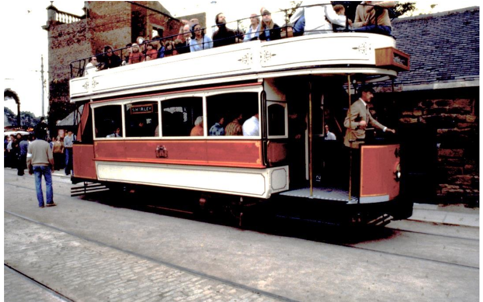
Southampton No. 45 features "knifeboard" seats on its open upper deck. The tram, built in 1902 by Hurst Nelson, single-handedly launched the tramway preservation movement in Britain since it was the first car purchased by enthusiasts. (Richard Thompson photograph)
