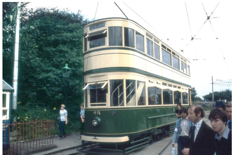
Blackpool No. 49 was built in 1926 using a few parts inherited from a predecessor built by Hurst Nelson in 1902. The top was covered in the late 1920s and the vestibules and balconies enclosed a few years later in 1930. (Richard Thompson photograph)
