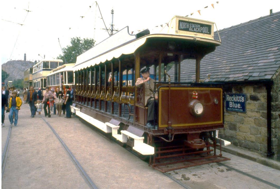
Blackpool & Fleetwood No. 2 is a relatively high capacity single deck "toast-rack" car that was built in 1898 for service on the line between Blackpool and Fleetwood. It was well-suited to the interurban-like route, which opened that year. (Richard Thompson photograph).
