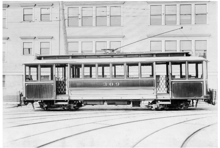
The first Fuller Standard cars were created in 1902 by adding large platforms and a second truck to old single-truck Pullmans.
