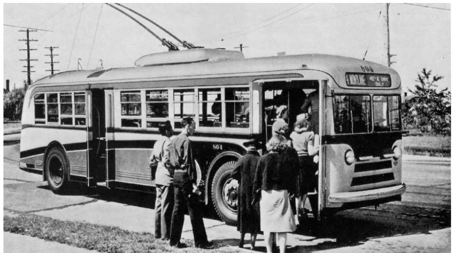
Seattle's first Twin Coach trolleys, numbers 800-934, arrived in 1940. They were powered by a 125 hp Westinghouse motor giving a speed of 40 mph. (Westinghouse photo)
