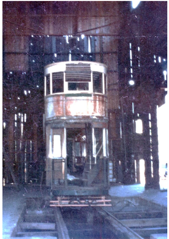
Blackpool double-decker No. 48 is being dismantled for restoration. As can be seen, part of the vestibule has been removed at one end.
