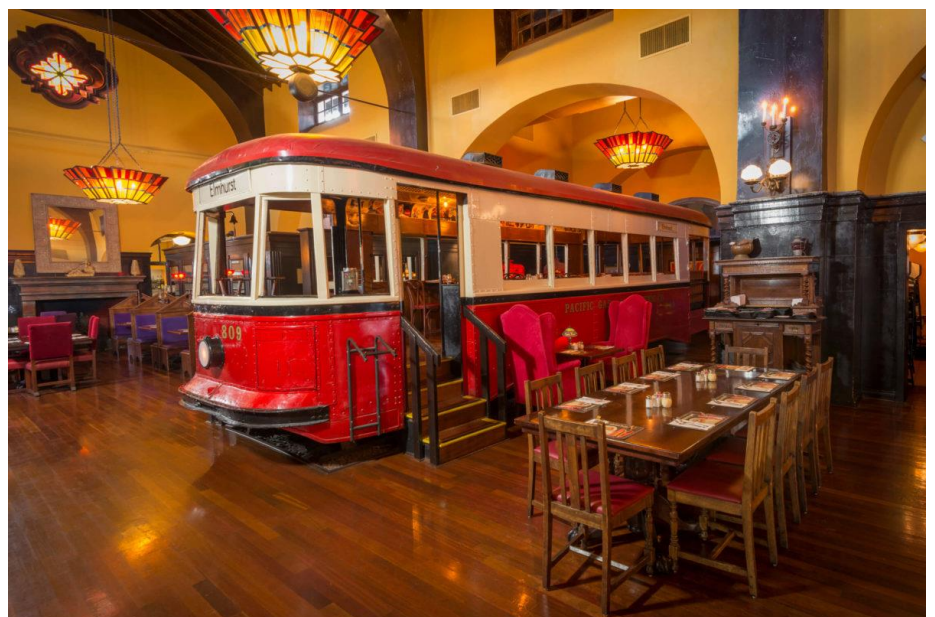
No. 809, now ensconced in the Sacramento Old Spaghetti Factory, resembles a Birney Safety Car more than a Brill Master Unit because ten feet had to be removed from the center of the car so that it would fit inside the restaurant. (Old Spaghetti Factory photograph)
