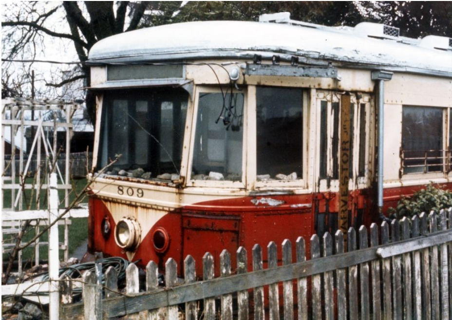
The stop lights on No. 809 are clearly in view in this snapshot taken a short time before the car was moved from a yard in Aurora, Oregon where it was used to store a rock collection. These lights were among parts salvaged from the former Broadway car. (Thompson photograph)
